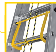
✓ HIGH RESISTANCE ! Two-arm locking system in steel tested to resist 350 kg (test 5.9 of EN 131).
