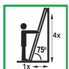
Lean the ladder with the correct slope against the wall. This can be easily checked by placing your feet in front of the ladder and using both horizontally held arms, holding the ladders by the beams.
