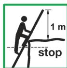
If you are using the ladder to access a roof, make sure that the ladder projects 1 m above the roof edge so that you have sufficient support when climbing up onto the roof. Do not climb higher than the roof edge to prevent the ladder from tipping over. If not sure, tie the ladder firmly or pin into the ground to secure the ladder base.
