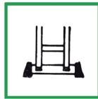
Never use the ladder without the base crossbeam. This must be installed before use.
