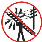
Watch out for electricity; a ladder is a life-threatening current conductor.
