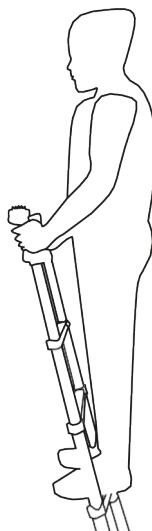
**12** Collapse the ladder after use by unlocking the bottom button with one hand, and pushing the ladder down with the higher-positioned other hand.
