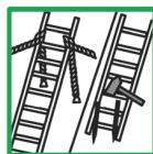
Ensure that the ladder is secured against slipping at all times. In case of doubt, tie the ladder firmly or pin into the ground to secure the ladder base.
