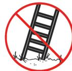
Place the ladder on a stable surface and make sure that it does not sink into the ground.
