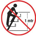
Never climb the top 3 rungs of the ladder. A ladder without protruding ladder ends or a ladder, in which some of the rungs at the top of the ladder are still collapsed (telescopic ladder), requires special attention and supervision to ensure that the top metre thereof is not climbed.
